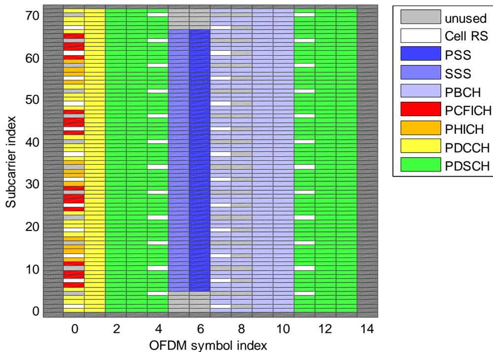
**Fig. 2** Downlink transmit resource grid for a sub-frame (1 ms)
