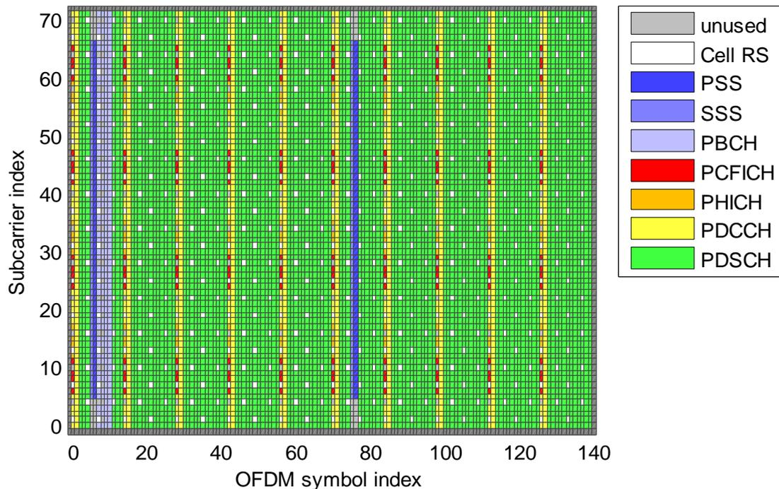
Fig. 3 Downlink transmit resource grid for a radio frame (10 ms)
