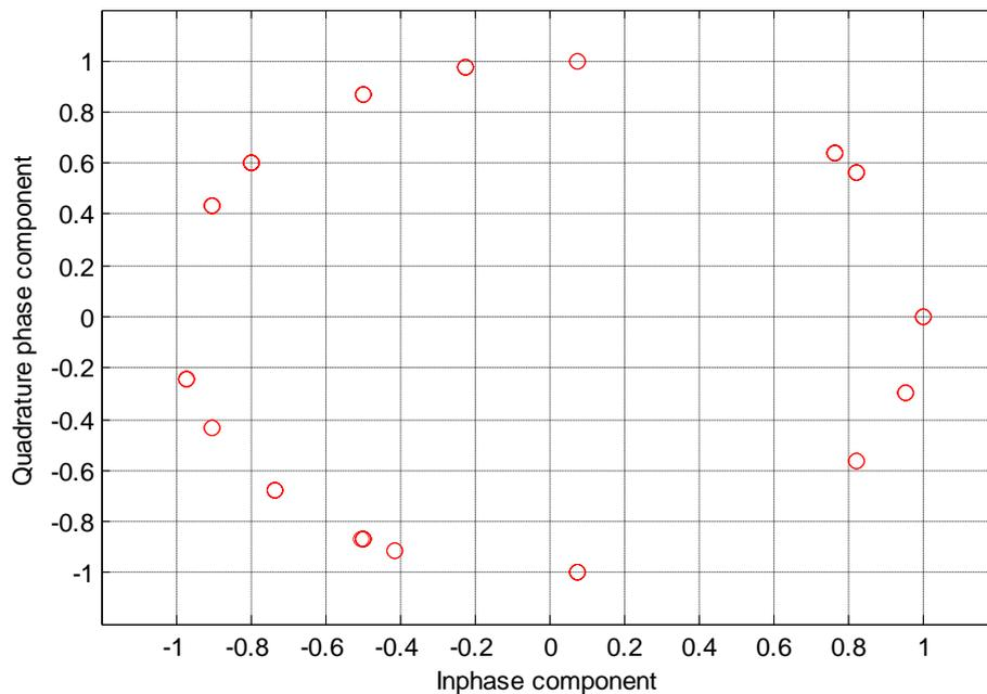
Fig. 1 Constellation diagram of Primary Synchronisation Signal
